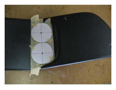
Once you're satisfied, mark the centers and drill one small pilot hole in each location (the pilot hole will help guide a hole saw if that's the tool you intend to
