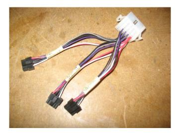
Prior to starting this however, it's good a idea to generate a wire list with circuit vs pin number to ensure no miswires, and then follow up with an ohm-out of each circuit using a multimeter. This is particularly true since each of the gauges shares the same color wires and can become confused for one another when assembling the harness. The last thing one would want is a short circuit on initial power-up. A sample wire list is below.
