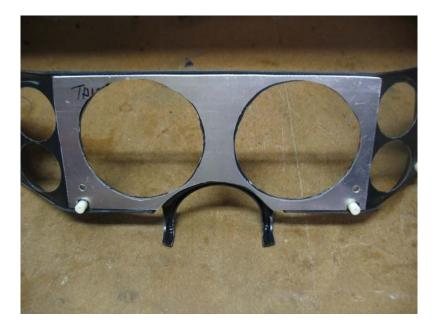
Now, the way I attached the bezel to the backing plate was to cover the entire mating surface with automotive grade double stick tape (after a thorough cleaning with isopropyl alcohol on both the backing plate and bezel). Set the backing plate on the workbench tape-side up, lay the bezel on top of it and press down hard across the entire area to ensure good adhesion. This backing plate will now provide some added rigidity to the bezel.
