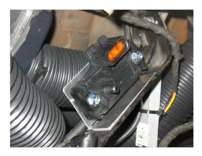
The MAP sensor may also be mounted inside the engine compartment. In which case like the oil pressure sensor, route a vacuum line to it from the engine and route the gauge wiring through a hole in the firewall using the grommet to protect the wires.
