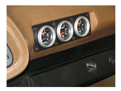
The last remaining things are to start the car and verify gauge operation as well as to calibrate the speedometer. If everything was installed correctly, you should have a beautiful, functional instrument cluster to enjoy!
