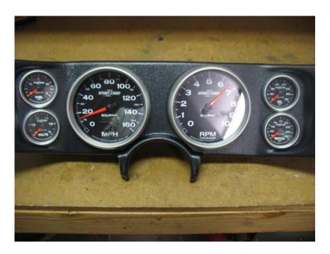
Clearly the 5" gauges leave very little material remaining. The bezel has been weakened too much to support the weight of the gauges and the stress of maneuvering the setup into the dash board. To remedy this, I made an aluminum backing plate. Here's how.
