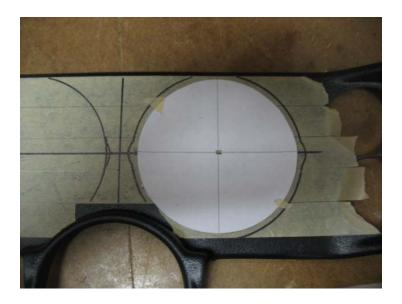
Now cut the holes. Again, a hole saw or a jigsaw can be used here. Once the holes are cut, test fit the gauges. The semi-completed Autometer/Covans instrument bezel should now look like this:
