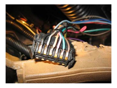
After soldering, it's recommended to coat the terminals in a silicone sealer and then wrap the connector in electrical tape to prevent shorts.
