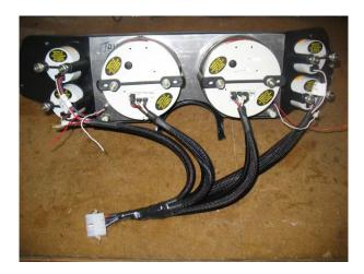
Populate the mating connector according to your wire list. At this point, it's recommended to take an ohm-meter and buzz out the wire harness with a point to point check. This will insure that you've populated the connector correctly and will prevent miswires resulting in possible damage to the hardware.
