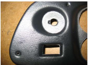
Moving on to the 5" gauges, I used the gauge retaining brackets to simulate the outer bezel diameter of the gauges themselves (it's very close). Placement of these is somewhat a matter of preference, but be sure to place them such that there is as much material remaining on either side as possible.
