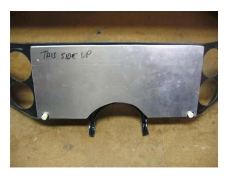
Once the backing plate fits properly against the bezel, mark the 5" gauge holes from the front. Remove the backing plate and then cut the holes with either the hole saw or the jig saw.
