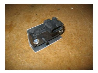
Finally, with some automotive grade double stick tape, the assembly was fastened to a bracket under the dashboard and the previously existing vacuum line was routed to it.
