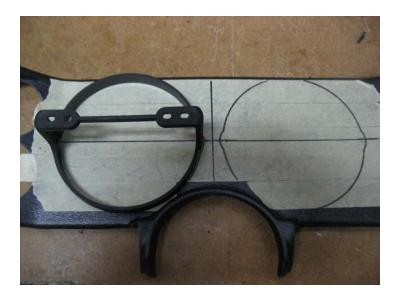
Then using the same paper template method, locate the exact centers of the holes.
