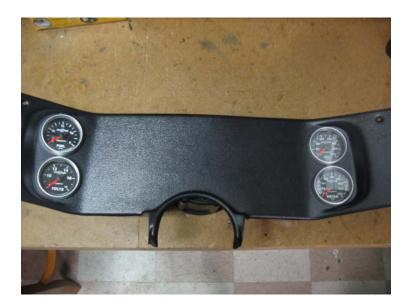
Remove the gauges and locate the area for the headlamp switch and wiper switch. Drill out the hole for the head lamp switch retaining nut. Also, using a razor knife carefully cut away the rectangular opening for mounting the wiper switch.
