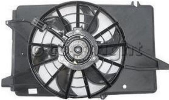
Try to get one with a large integral shroud so as to cover as much of the radiator as possible. Your low vehicle-speed cooling ability (particularly stopped at idle) hinges on maximizing air flow through the radiator. The more shroud area, the greater the ability of the fan to pull air through the radiator.
