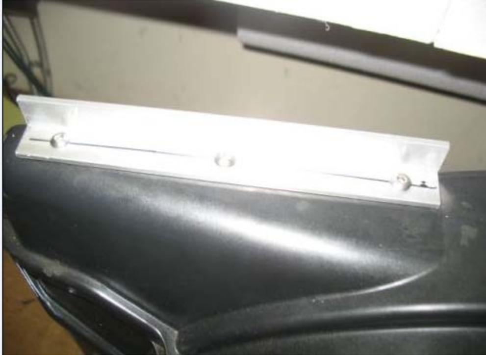
Since the fan has mass and will be under constant vibration loading while the car is in motion, using this type of angle bracket scheme across the top of the fan shroud will spread the load across a wide patch of the plastic shroud to minimize stress.
