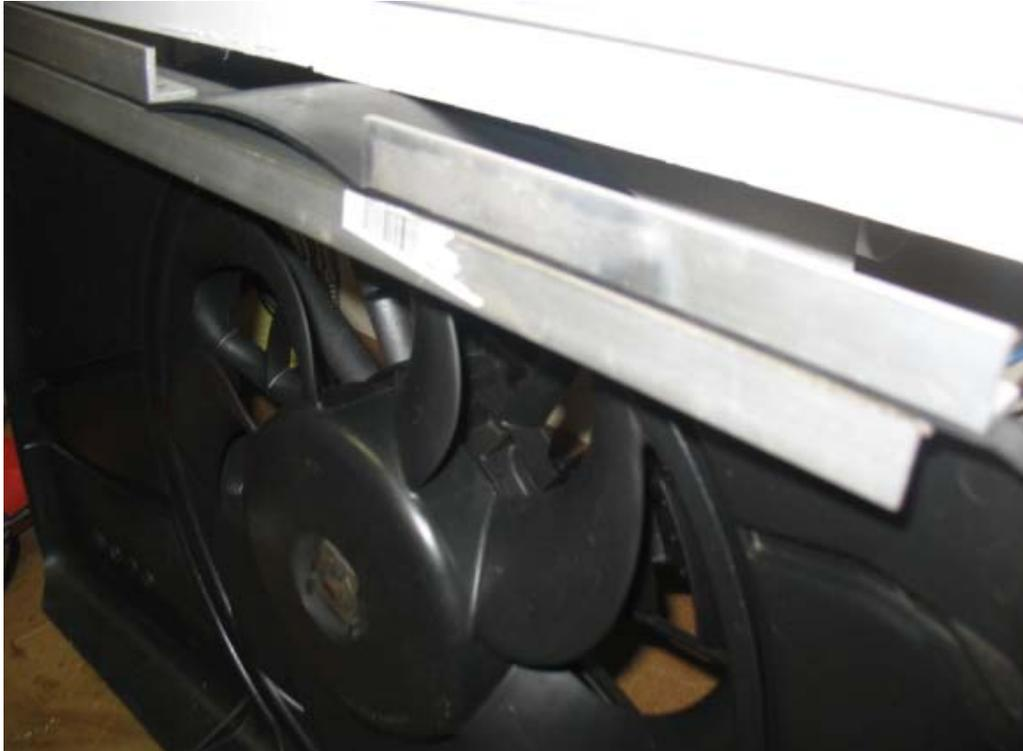
In the above photo, note how I have the aluminum angle sandwiching the plastic shroud. The flat part of the angle should be approximately flush with the edge of the shroud. The angle pieces are then fastened together with locking fasteners per the picture below. Simply drill through the top angle, the shroud, and the bottom angle and then run fasteners and locking nuts. Use locking nuts to prevent the fasteners from loosening up over time.
