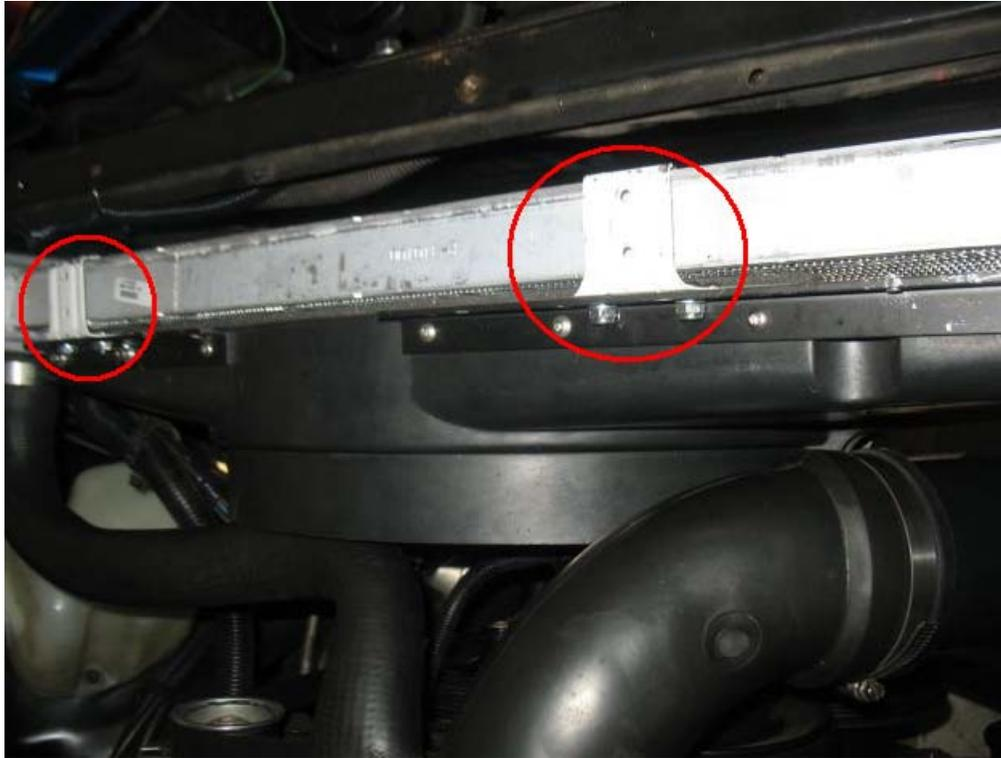
Below is a close up of the U bracket installed. Note the aluminum angle has been painted flat black. The U bracket bolts to the aluminum angle. Use as low a profile screw head as possible since the screw head is on the radiator side.
