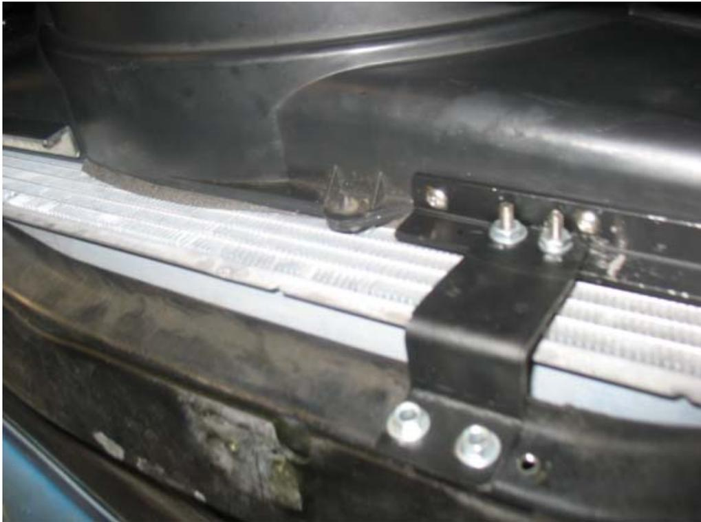
With the shroud fastened to the radiator, now it's just a matter of putting the top radiator cover on.
